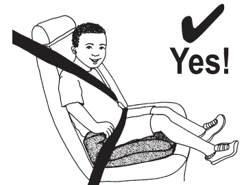
A booster helps the seat belt fit properly. This is a backless booster.
