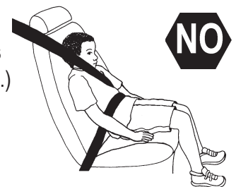
Poor seat belt fit. Child is too small to use it safely.
